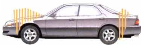
The front and rear crumple zones are designed to progressively give upon impact, rather than directly pass the energy on to the driver and passengers.
